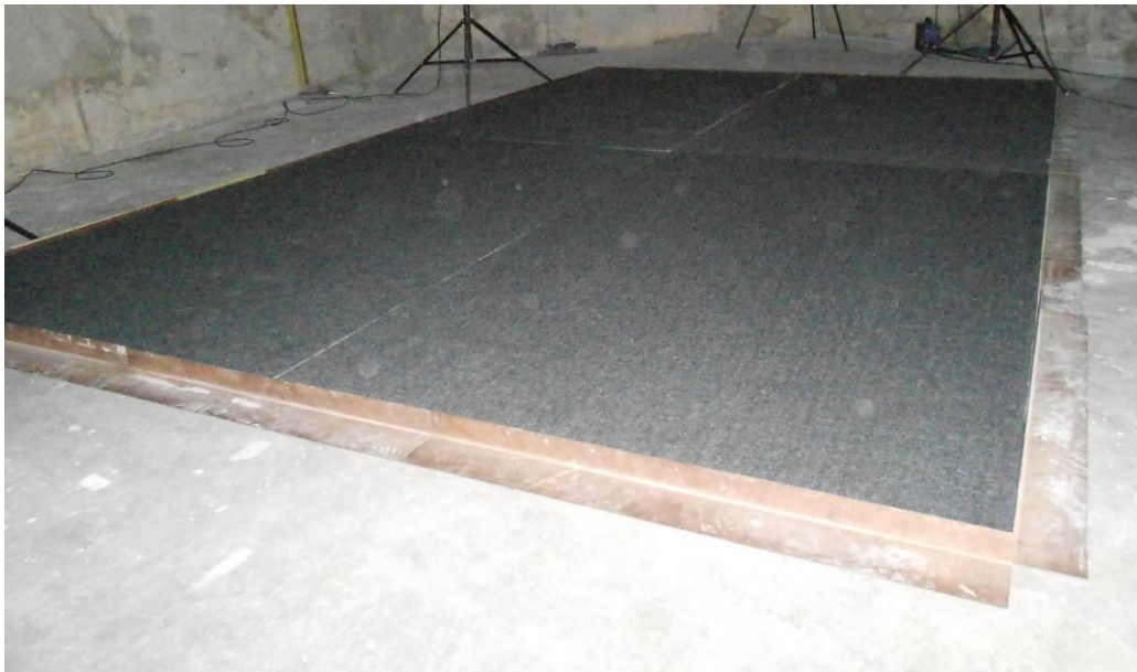
Figure 2: Echo Panel 24mm tested with a 20mm air gap installed in Reverberation Chamber
